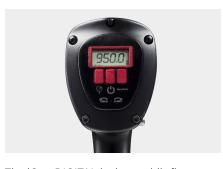
The jGun DIGITAL is the world's first torque-adjustable pneumatic multiplier with a digital readout and FRL-free operation. Unlike other systems that require a separate filter, regulator and lubrication system, the patented design of the jGun DIGITAL eliminates the need for this add-on for the highest level of portability and convenience.
