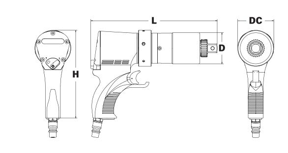
**LEGEND:** H = HEIGHT L = LENGTH D = OUTER DIAMETER OF GEARBOX DC = DIAMETER OF COLLAR
